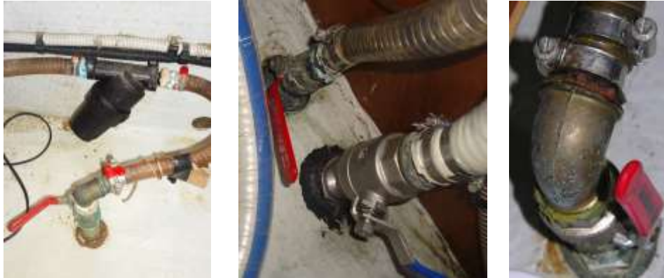
Air-con intake seacock and strainer concerns – Mixture of metals concerns
